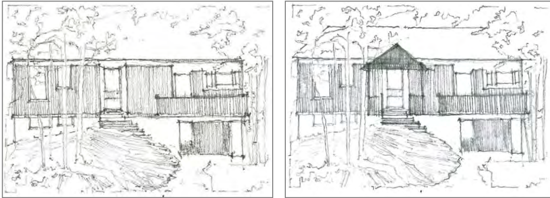
Figure 36: The sketch on the left illustrates an existing flat roofed house. The sketch on the right illustrates an inappropriate alteration to the original building (addition of a gable roof).
